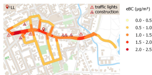
Fig.1 Wintertime distribution of BC in the City of Leipzig as measured with mobile sensor. After Alas et al., 2019.
